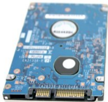
SATA drive (has card-edge connector)
