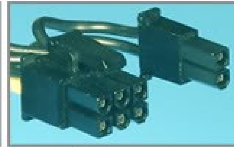
PCI-E Connector 8 (6+2) Pin
