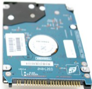
PATA drive (has pin connector)
